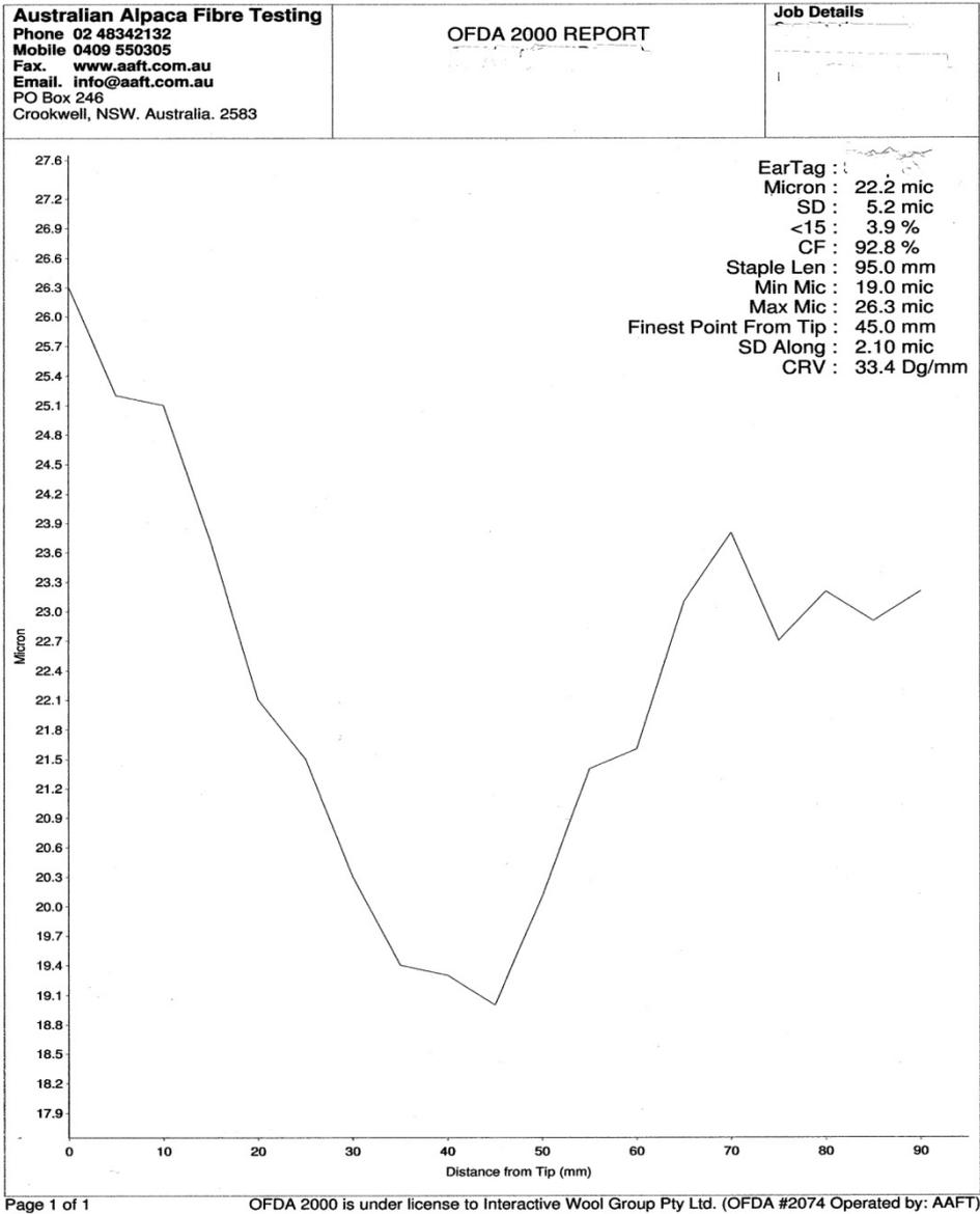
Figure 4 Fibre diameter profile as measured by OFDA2000
