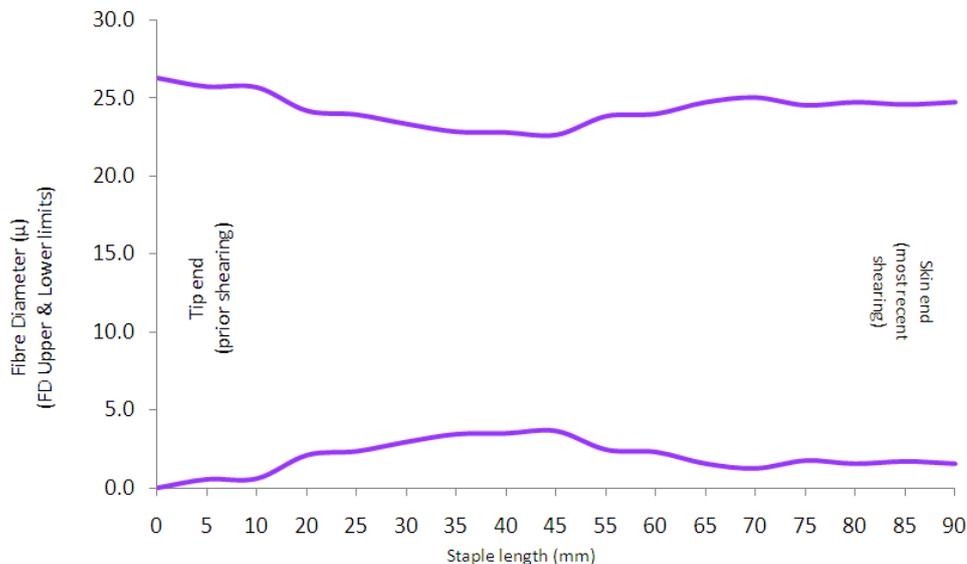
Figure 3 Fibre diameter profile average showing extreme variation along the fibre length
